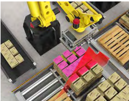
Robot-mounted Gocator 2490 used for depalletization
